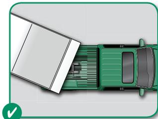
The Husky 16K Roller is designed to allow the 5th Wheel hitch assembly to move up to 9" rearward, which opens up the distance between the nose of the trailer and the rear window/cab of the pickup, and allows tight maneuvering without contact or damage.
